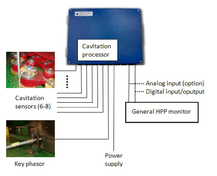
Cavitation Monitoring System Korto 7391 Used as a cavitation channel of the general HPP monitoring system Cavitation data are delivered as digital or, optionally, as 0/4-20 mA analog.
