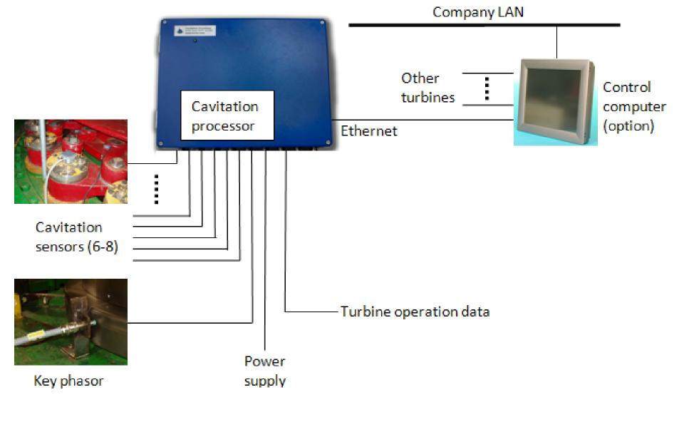
Cavitation Monitoring System Korto 7391 Cavitation data from all units are concentrated in the control computer, optionally. Real-time cavitation data displayed to operators; logging in the company server
