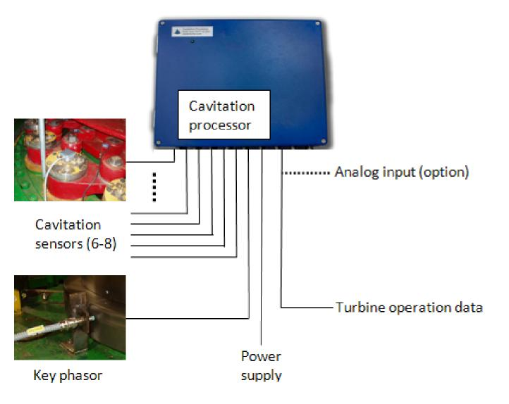
Cavitation Monitoring System Korto 7391 Analog operation data input, optionally Up to 6 channels; 0-20 mA, 4-20 mA, 0-10 V selectable
