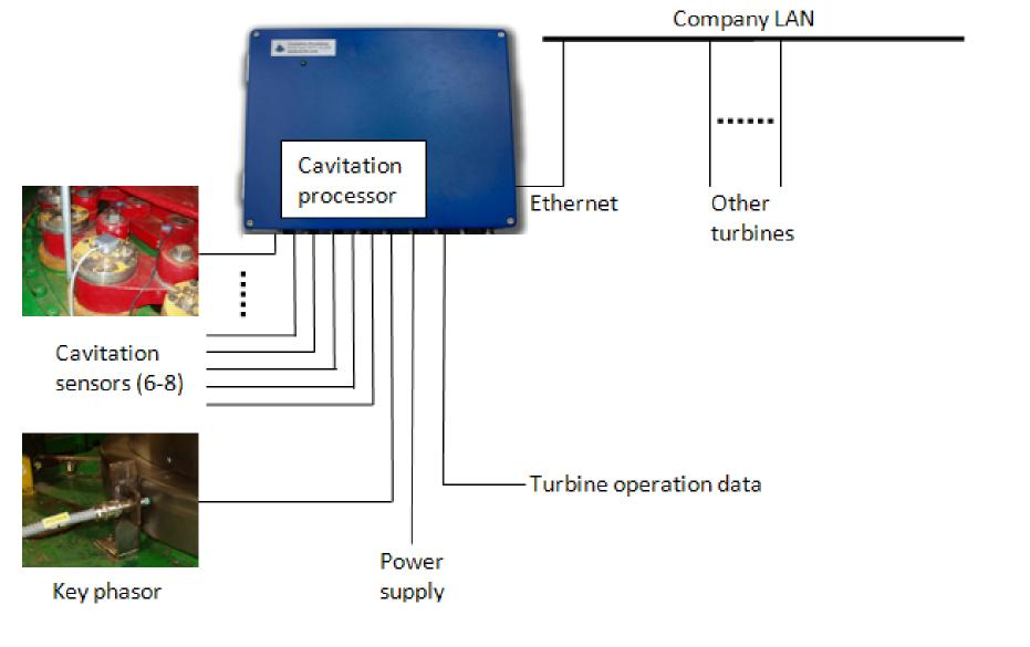
Cavitation Monitoring System Korto 7391 Independent use – Cavitation data delivered directly to company LAN Logging in the company's server, users' PCs connected via LAN
