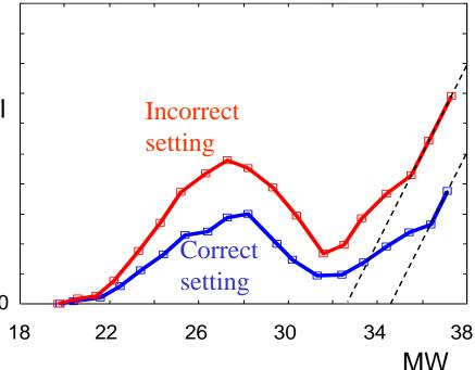
The multidimensional cavitation monitor distinguishes between turbine parts. It delivers independent estimates of the intensity of cavitation close to each runner blade. Thus, the small initial change is not compared to the total intensity of all the blades but, instead, to the intensity of the damaged blade only. This makes the monitoring sensitivity higher by a factor equal to the number of runner blades.
