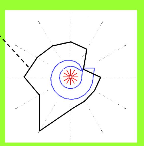
The estimate of the mean total cavitation intensity strongly depends on the position of the sensor with respect to the spiral casing.
